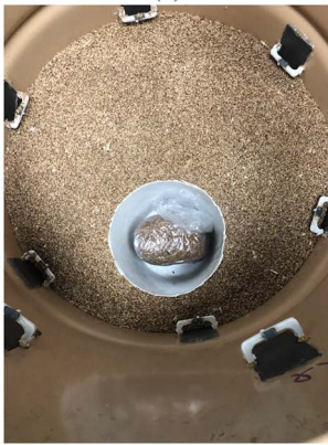
FIGURE 8. (a) Exterior photograph of the barrel with the VNA/switch connected to all 24 antennas. (b) Schematic diagram of model grain bin. (c) Image of the wet-grain target with marker for scale. Images of the interior of the barrel are shown in (d) and (e). Grain was filled with a wet grain mixture covered in plastic in a bucket. (d) Dry grain is placed in the bucket then (e) we covered up to the wet grain mixture and leveled the grain.
