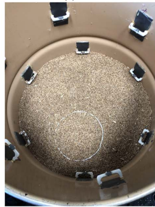
FIGURE 8. (a) Exterior photograph of the barrel with the VNA/switch connected to all 24 antennas. (b) Schematic diagram of model grain bin. (c) Image of the wet-grain target with marker for scale. Images of the interior of the barrel are shown in (d) and (e). Grain was filled with a wet grain mixture covered in plastic in a bucket. (d) Dry grain is placed in the bucket then (e) we covered up to the wet grain mixture and leveled the grain.
