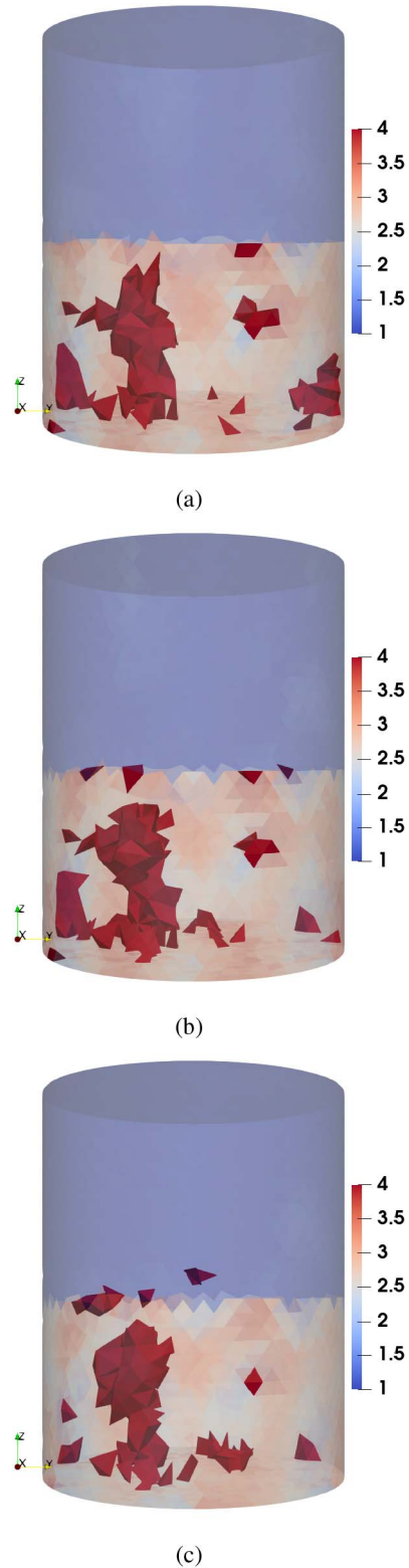
FIGURE 15. One-shot Calibrated Experimental FEM-CSI inversion 3D images of Re(\epsilon) with a threshold at the frequencies of (a) 550MHz, (b) 560MHz, and (c) 570MHz. All tetrahedrons beyond a threshold of 4 are solid.
