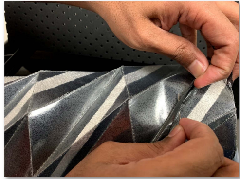
FIGURE 32. Folding appropriately and then hand-stitching the edges to form the desired origami Kresling pattern.
