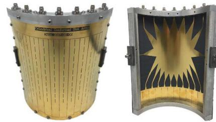
FIGURE 11. Conformal SIW-based dual-layer Rotman lens [53].
