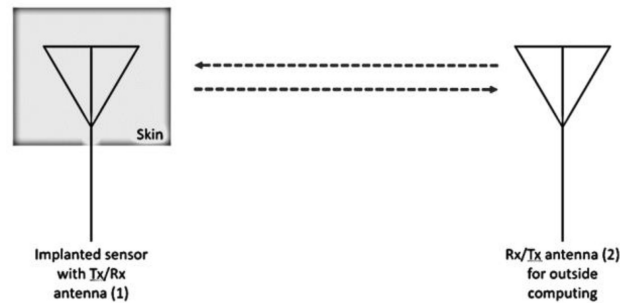
FIGURE 7. Experimental set up for implantable sensor communication with fabric antenna (CKA).
