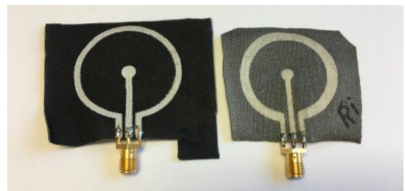
FIGURE 14. (Left) Fabric antenna (CKA) W/ interface layer. (Right) Fabric antenna (CKA) W/O interface layer.
