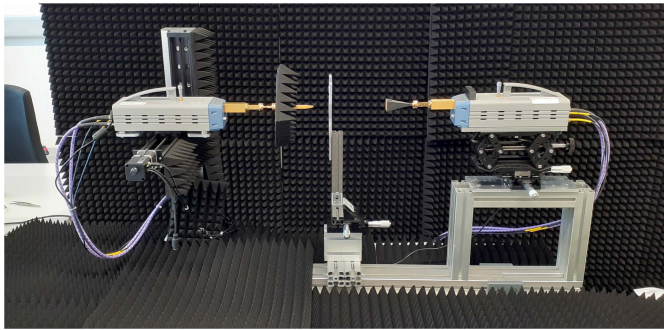
FIGURE 3. Near-field scanning setup with standard horn antenna exciting the mm-wave lens.
