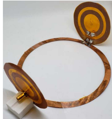
FIGURE 3. Prototype of the proposed CSCMR system with a simplified U-loop.
