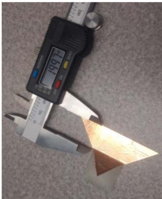
FIGURE 1. BMA with a conducting flare extension to improve the low frequency cutoff.
