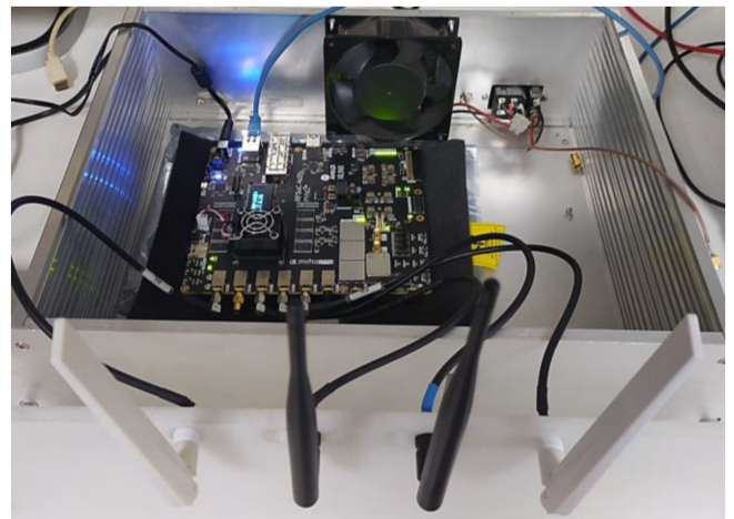
FIGURE 9. Rack with RFSoc and experimental antenna elements for coupling coefficient measurements C_{mk} and C_{km} .
