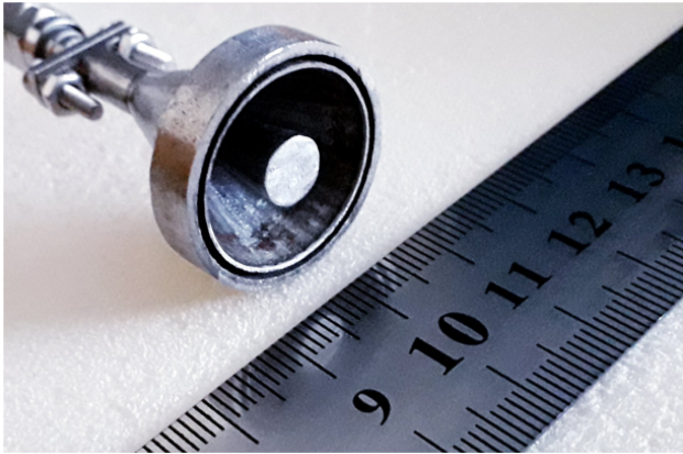
FIGURE 11. Photograph of the fabricated coaxial horn antenna placed next to a ruler with millimeter and centimeter graduations.
