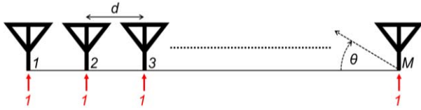
FIGURE 1. Uniform M -element antenna array.
