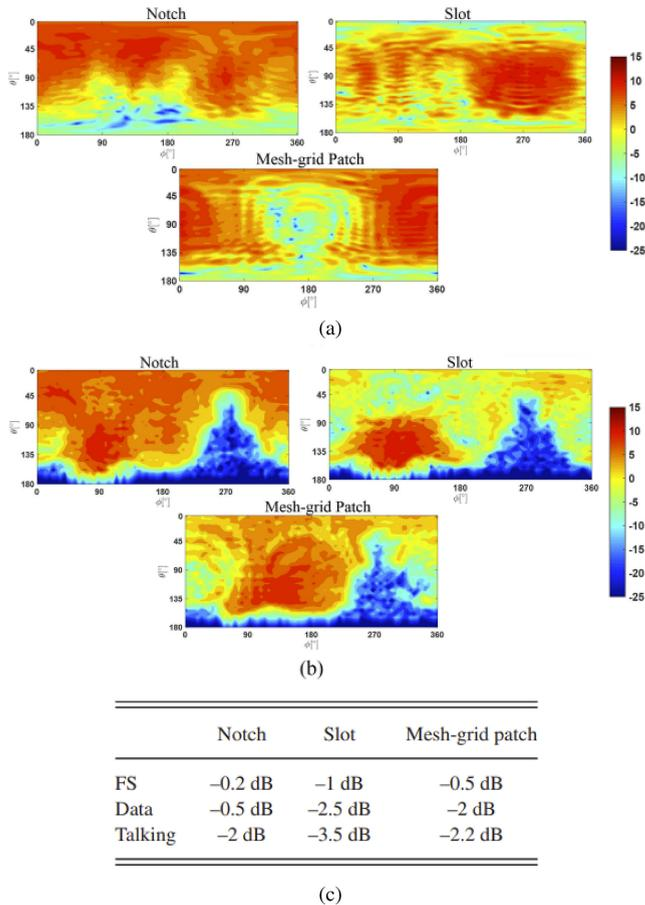
**FIGURE 8.** Radiation pattern of antennas in free space in (a), with the user in (b), and the measured body loss of different antennas in (c) [30].
