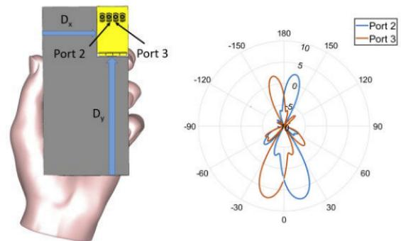
**FIGURE 12.** The proposed phased antenna array location in and radiation patterns for two ports on the antenna [12].
