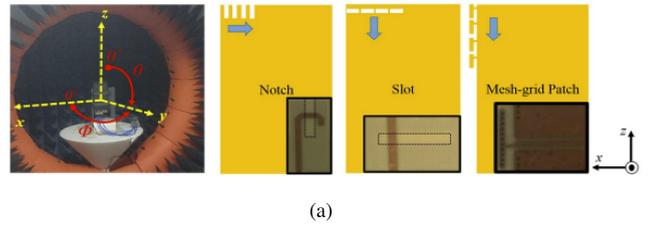
FIGURE 7. Measurement setup in free space in (a) and with the user in (b) [30].
