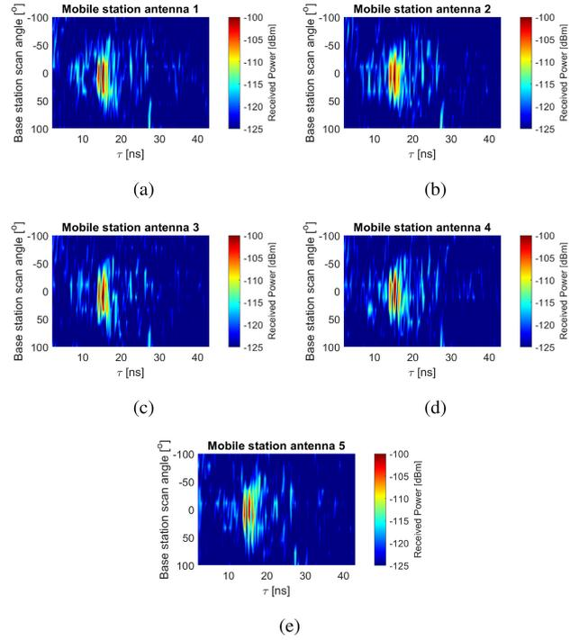
**FIGURE 21.** An example of angular delay profiles of the corridor propagation channel with the user in front position and the mobile station array located on top measured with (a) antenna 1, (b) antenna 2, (c) antenna 3, (d) antenna 4, and (e) antenna 5.
