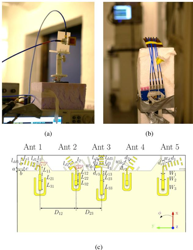
**FIGURE 18.** Horn antenna base station setup in (a), mobile station setup with an RF switch in free space in (b) and the 5G yagi-uda antenna used in the measurement campaign as a smartphone mobile station mock-up in (c) [49].
