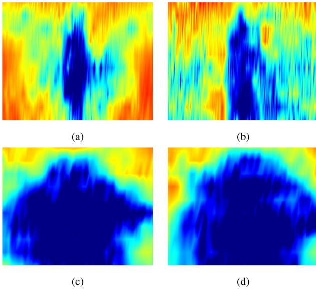
**FIGURE 14.** Image of the radiation pattern of the user with full antenna radiation pattern (a) top antenna and (b) bottom antenna, and the radiation pattern of the shadow region (middle  $\pm 45$  degree) for (c) top antenna and (d) bottom antenna.
