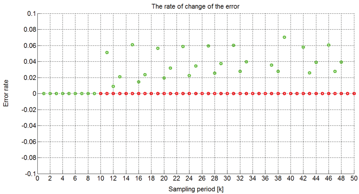
Figure 16: Rate of change of the error for observer initial conditions of 1.0 and model initial conditions of 1.0 using a constant control input of 1.0.
