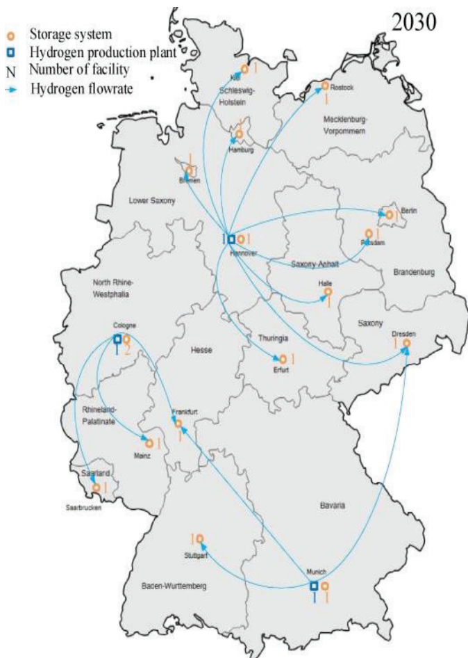
Fig. 1: The GH transportation infrastructure for 2030 [18].
