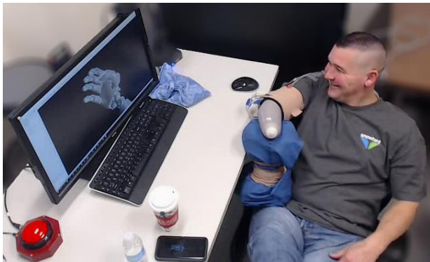
Figure 1: Training and testing of real-time proportional six-DOF motor-decode algorithms for a virtual prosthetic hand. This participant had undergone a transradial amputation of his right hand 5-6 months prior to experimental sessions, due to long-term complex regional pain syndrome (CRPS) and disuse of the affected hand. At the time of surgery, the participant also received implants of three 100-electrode USEAs in his residual arm nerves proximal to the elbow, plus a 32-channel assembly of electromyographic (EMG) electrodes in his residual extrinsic hand muscles in his forearm. The implanted devices allowed recordings of neuromyoelectric signals during subsequent experimental sessions. EMG recordings were obtained from the two intact subjects with temporary surface EMG electrodes. During training sessions, participants mimicked the movements of the virtual hand with their phantom hand (amputee participant) or intact hand (two intact participants). During subsequent testing sessions, participants attempted to reach and hold a target position (0.5 of full flexion) for a particular DOF while maintaining all other DOFs at their resting positions.
