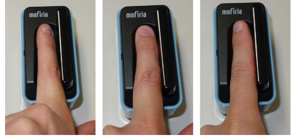
Fig. 2. Finger rotation example using a commercial off-the-shelf scanner (rotation counter-clockwise, originally published in [3]).
