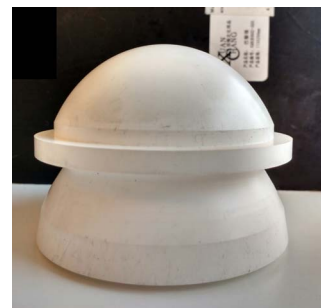
Fig. 1. Machined Preperm lens. The diameter of the lens is 64 mm.
