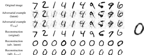
Fig. 4. Summary of different attacks on MNIST dataset and VAE-GAN model: original images, adversarial examples for both methods (latent and \mathcal{L}_{VAE} ) and reconstructions of original images and adversarial examples. Target reconstruction is shown on the right.
