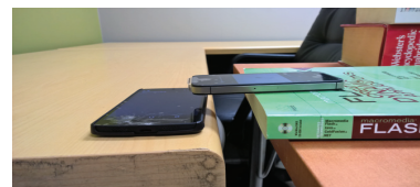
Fig. 3: Experiment setup depicting a phone speaker against the smartphone with embedded motion sensors that are placed on different surfaces .
