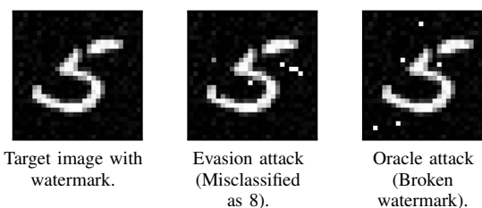
Figure 1. Examples of attacks against machine learning and digital watermarking. Middle: the target is modified, such that it is misclassified as 8. Right: the target is modified, such that the watermark is destroyed.
