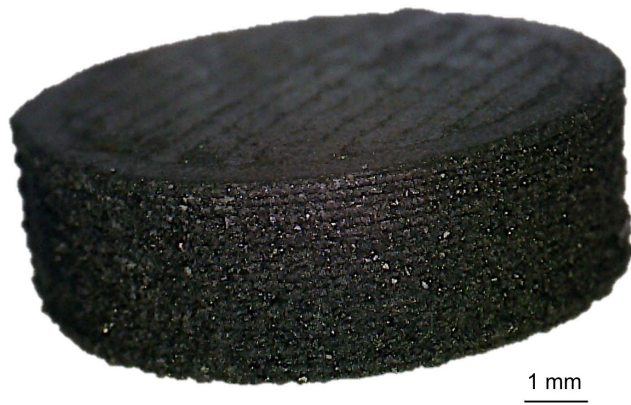
Fig. 5. An example of a finely FFF-printed magnet using filament made of pellets of the compound RNI-40LF. Individual 150\ \mu\text{m} -thick layers are visible on the side of the printed object, as well as 600\ \mu\text{m} -wide strips on its top.
