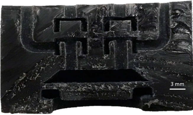
Fig. 6. Example of a diaphragm pump 3-D printed in one piece of a TangoBlack ® blend with Shore 50A hardness. The device was cut with a razor blade after printing and post-cleaning of the sacrificial material that filled-in the cavities.
