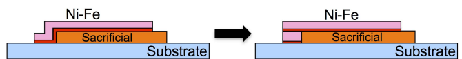
Fig. 13. Modification of the single step electroplating of a Ni-Fe cantilever to a two-step scheme.
