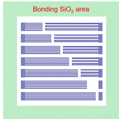
Fig. 5. Stiction test patterns.
