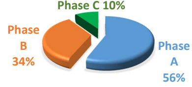
Figure 3. Distribution of voltage sags per phase in a 3-year PQ survey in Brazil [17].
