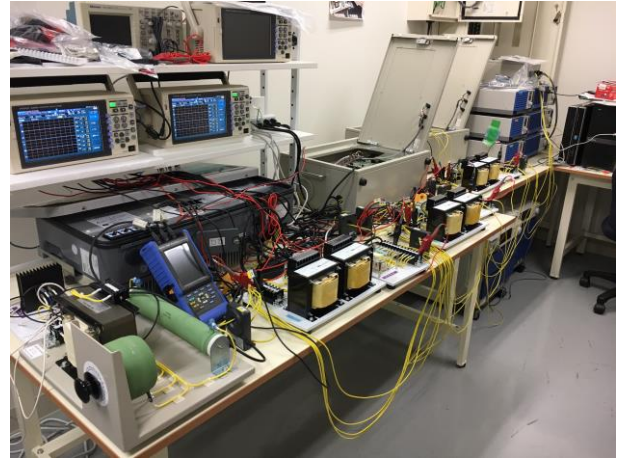
Figure 7. Simulated distribution system equipment.
