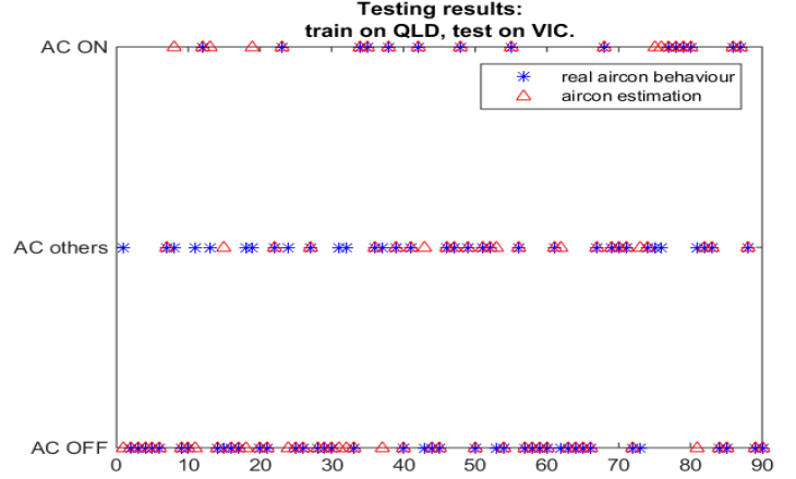
Figure 2. Classification of the days, training with summer days in QLD Queensland, and test testing on 90 summer days in VIC Victoria
