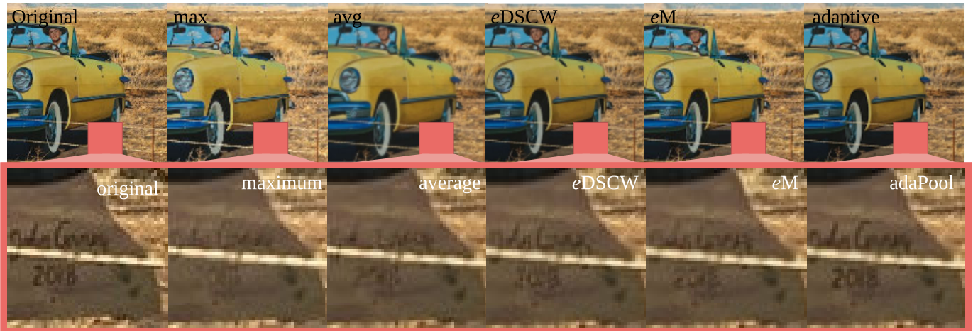
Fig. 3. Example of detail preservation with different pooling methods. Common methods such as average and maximum pooling result in a distorted signature with unrecognizable details such as numbers or characters. Exponential weighting through either normalized local maximum ( eM ) or similarity-based measures ( eDSCW ) better capture details. Further improvements in the detail and representation quality are observed when introducing an adaptive fusion between both of these exponential weighting methods ( adaPool ).
