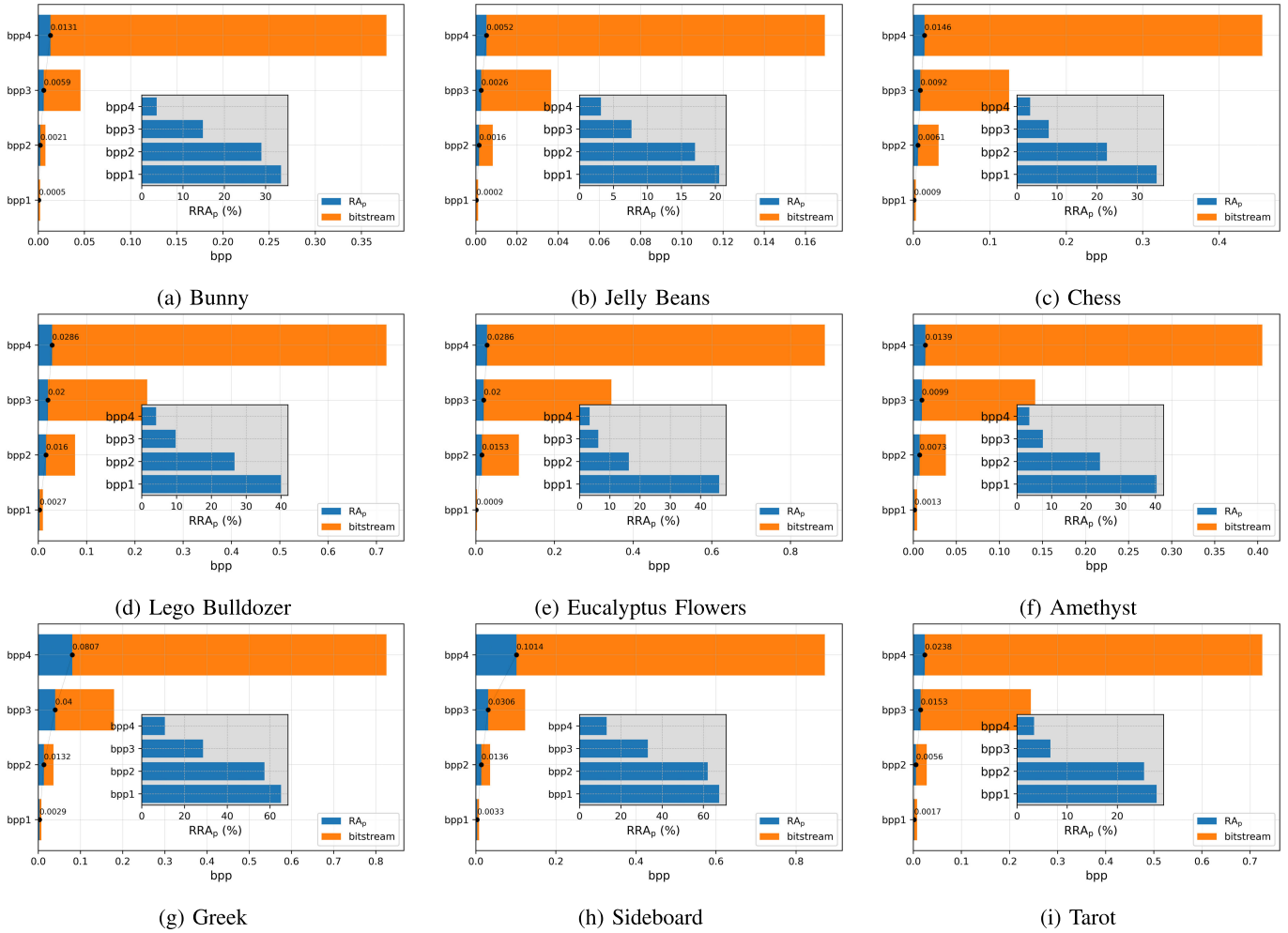
Fig. 12. RA_p and RRA_p for light field test images. RA_p denotes the maximum number of encoded bits required to access an arbitrary view at each bitstream. The embedded plots represent RRA_p , i.e., the relative number of encoded bits required to access an arbitrary view at each bitstream.
