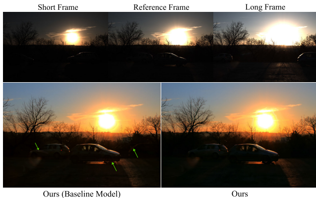
Fig. 8. Qualitative evaluation of our model on a test scene from the Tursun dataset with multiple fast moving objects which are present in all input frames. The baseline model struggles with ghosting artefacts, indicated by the green arrows. Our method is able to eliminate these artefacts entirely.
