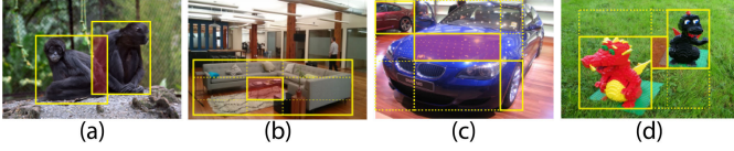
Fig. 4. Generalized Intersection Box (shown in red). (a) When two bounding boxes partially intersect, the generalized intersection box is the same as the intersection box. (b) When a smaller bounding box is completely inside a larger bounding box, the generalized intersection box is the same as the smaller bounding box. (c) and (d) When two bounding boxes do not intersect, the generalized intersection box is formed using the second and third smallest x coordinates and y coordinates of the two bounding boxes.
