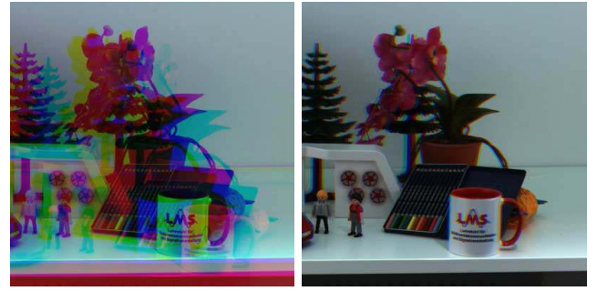
Fig. 5. Recordings of the images \{I_5, I_c, I_3\} lead to a color image. On the left-hand side, the color components are not calibrated and suffer from a depth-dependent shift. On the right-hand side, the channels have been rectified. Consequently, the color channels are aligned for the calibrated depth plane in the background. The remaining shift in color channels results due to the horizontal disparity of the cameras.
