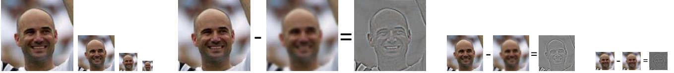
Fig. 4. Training data generation. The figure shows (from left to right): an example of the training image quadruplets generated with Guassing blurring and decimation, residual images at three different spatial resolutions (corresponding to the residuals added by the 8\times , 4\times and 2\times super-resolution steps). Note that the residuals are generated by subtracting a blurred version of the reference image at the given resolution from the original reference image.
