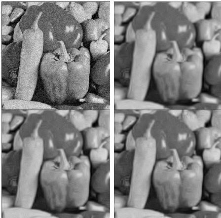
Fig. 8. Denoising example. Clockwise from upper left, noisy image ( \sigma = 20 ), OMP denoised, L-POMP denoised, OT-POMP denoised with DCT dictionary, k = 1 .
