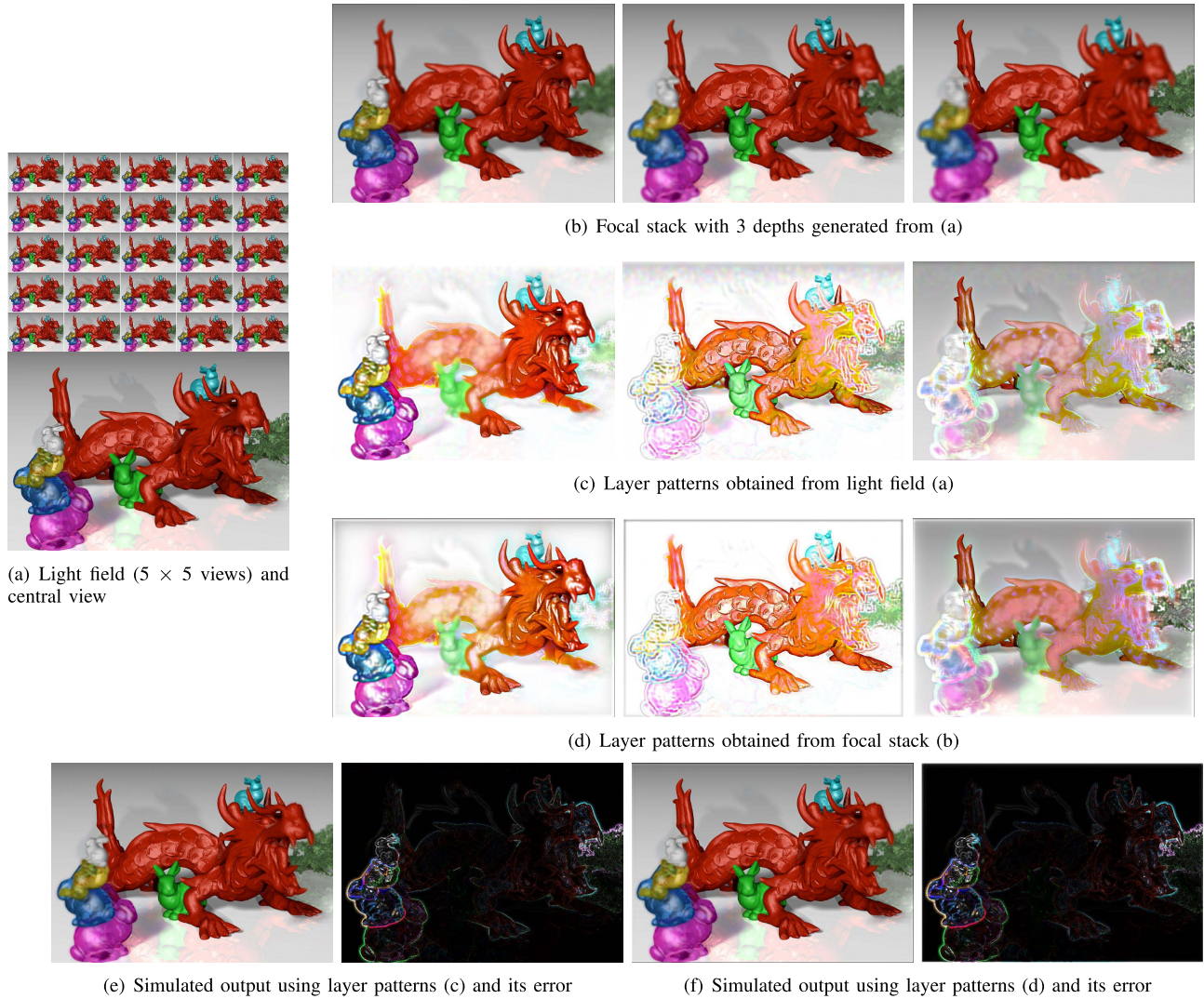
Fig. 8. Overview of experiment with synthetic light field dataset. From light field dataset (a), we generated focal stack (b). Layer patterns obtained from the light field and focal stack are shown in (c) and (d), respectively. Simulated outputs, which were computed from layer patterns in (c) and (d), are visualized in (e) and (f), respectively.
