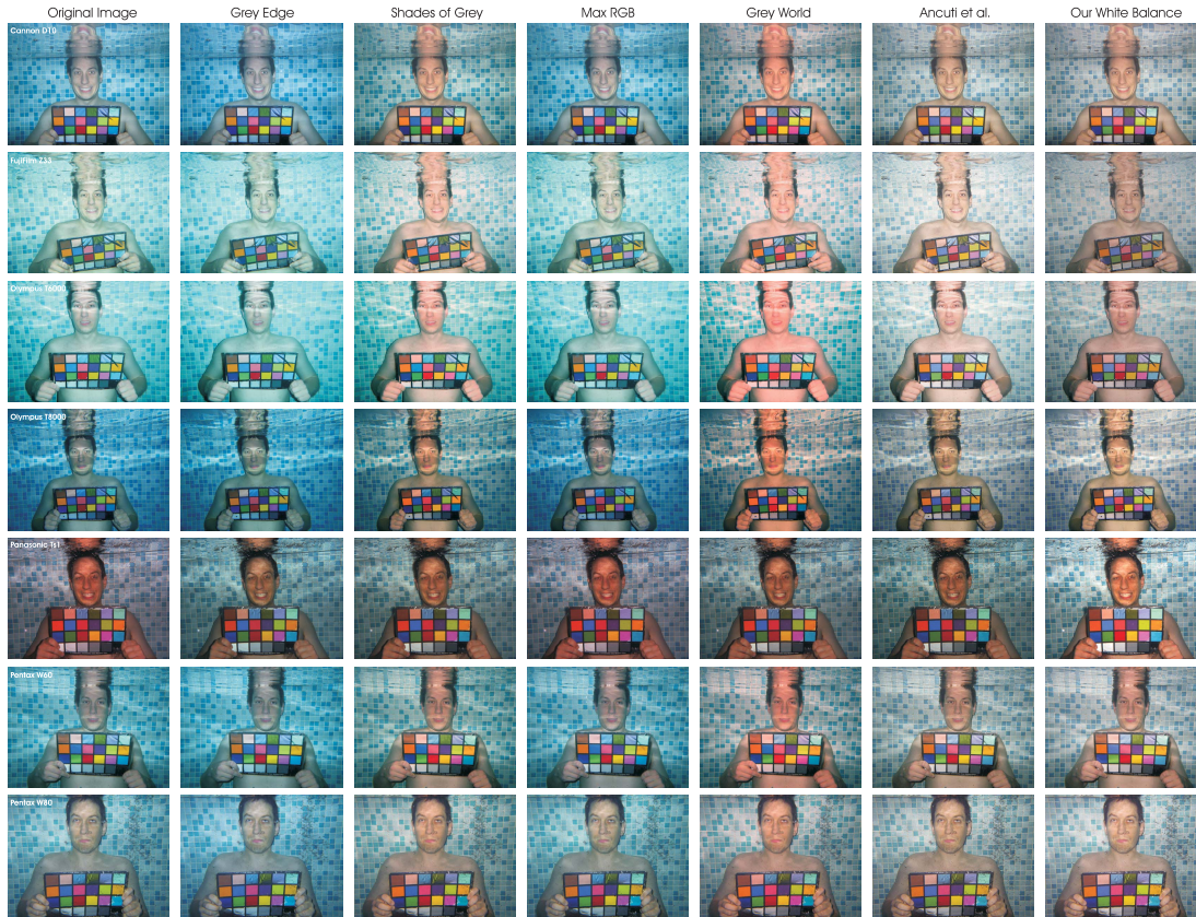
Fig. 9. Comparative results of different white balancing techniques. From left to right: 1. Original underwater images taken with different cameras; 2. Gray Edge [40]; 3. Shades of Gray [41]; 4. Max RGB [42]; 5. Gray World [43]; 6. Our previous white balancing technique [35]; 7. Our new white balancing technique. The cameras used to take the pictures are Canon D10, FujiFilm Z33, Olympus Tough 6000, Olympus Tough 8000, Pentax W60, Pentax W80, Panasonic TS1. The quantitative evaluation associated to these images is provided in Table I.
