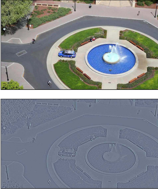
Fig. 3. Sample RGB (top) and pre-processed (bottom) input image, showing frame 61 from Neovision2 [27] Tower image sequence 001, which was first downsampled to a size of 960 \times 540 pixels. Image pre-processing involves the application of the whitening function used by Olshausen & Field [42], subtraction of the image mean and normalization of the result by its root mean square ( rms ).
