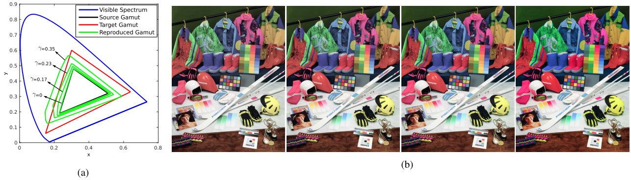
Fig. 2. Gamut extension approach. (a) Gamuts on chromaticity diagram. (b) Gamut extension results. From left to right: input image ( \gamma = 0 ), gamut extended image with \gamma = 0.17 , \gamma = 0.23 and \gamma = 0.35 . As the \gamma value increases the gamut becomes larger; notice the increment in saturation of helmets, socks, ski suits and shoes. Original image is courtesy of Kodak.
