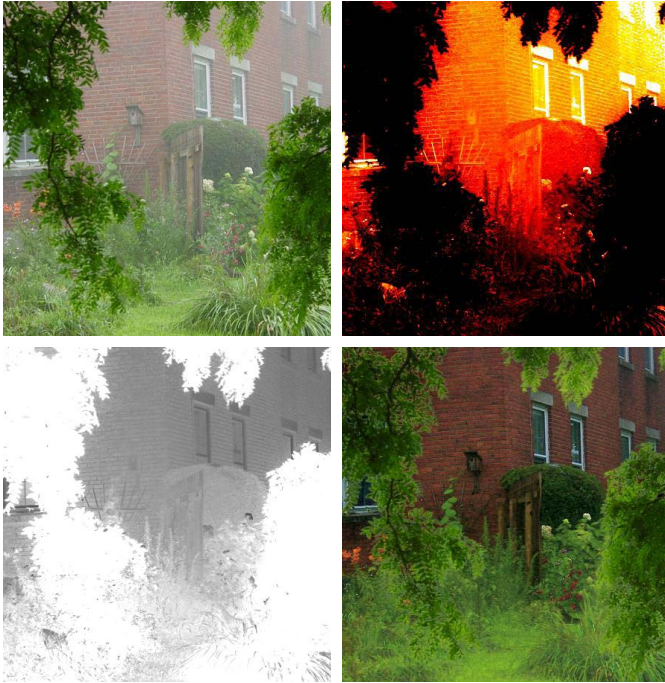
Fig. 1. An overview of the proposed dehazing method. Top-left: Input hazy image. Top-right: Restored depth map. Bottom-left: Restored transmission map. Bottom-right: Dehazed image.
