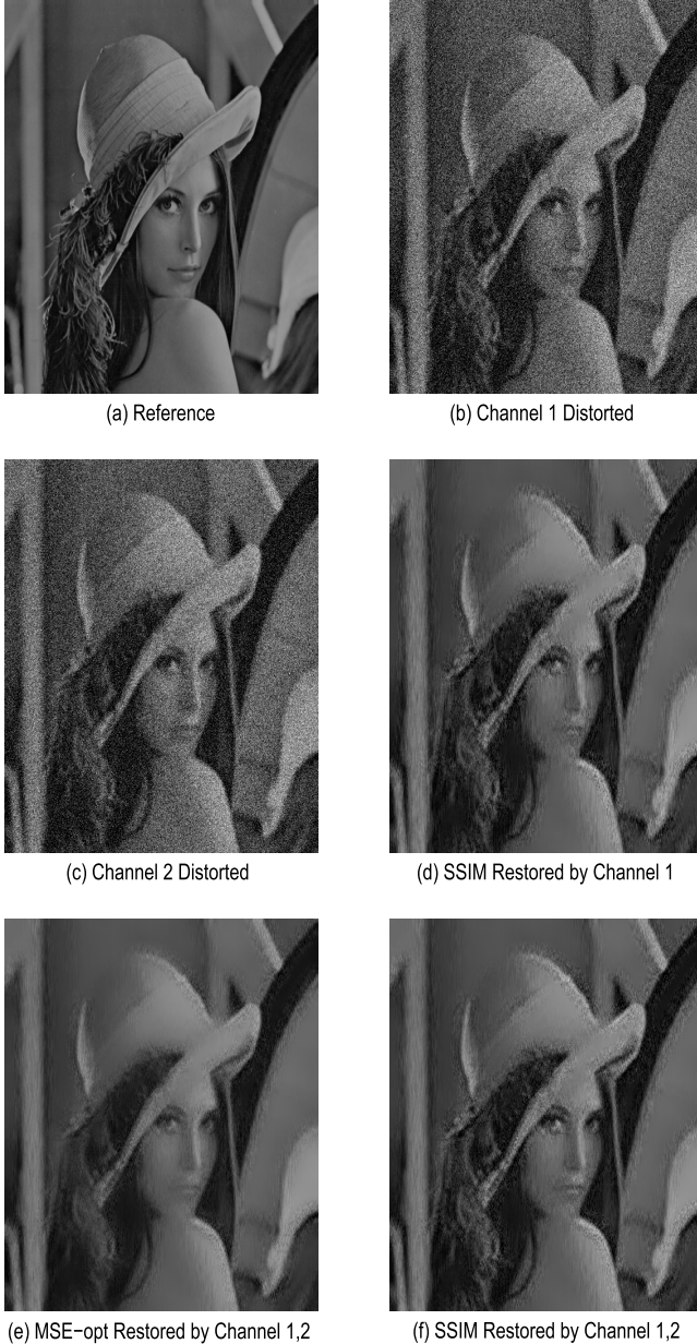
Fig. 13. Images restoration: (a) Original image. (b) Distorted image with \sigma_{H_1} = 2, \sigma_n = 35, \text{MSE} = 1273.888322, \text{SSIM} = 0.351978 . (c) Distorted image with \sigma_{H_2} = 3, \sigma_n = 35, \text{MSE} = 1280.202630, \text{SSIM} = 0.345316 . (d) Image restored with the SSIM-optimal filter by Channel 1, \text{MSE} = 226.380905, \text{SSIM} = 0.719319 . (e) Image restored with the MSE-optimal filter by Channel 1,2, \text{MSE} = 164.625729, \text{SSIM} = 0.716074 . (f) Image restored with the SSIM-optimal filter by Channel 1,2, \text{MSE} = 189.378151, \text{SSIM} = 0.761722 .
