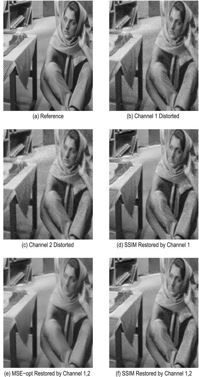
Fig. 12. Images restoration: (a) Original image. (b) Distorted image with \sigma_{H_1} = 2, \sigma_n = 25 , MSE = 899.902475, SSIM = 0.588095. (c) Distorted image with \sigma_{H_2} = 5, \sigma_n = 25 , MSE = 935.477916, SSIM = 0.571881. (d) Image restored by the SSIM-optimal filter of Channel 1, MSE = 628.557731, SSIM = 0.689969. (e) Image restored by the MSE-optimal filter of Channel 1,2, MSE = 499.992954, SSIM = 0.670820. (f) Image restored with the SSIM-optimal filter of Channel 1,2, MSE=609.016684, SSIM = 0.712847.
