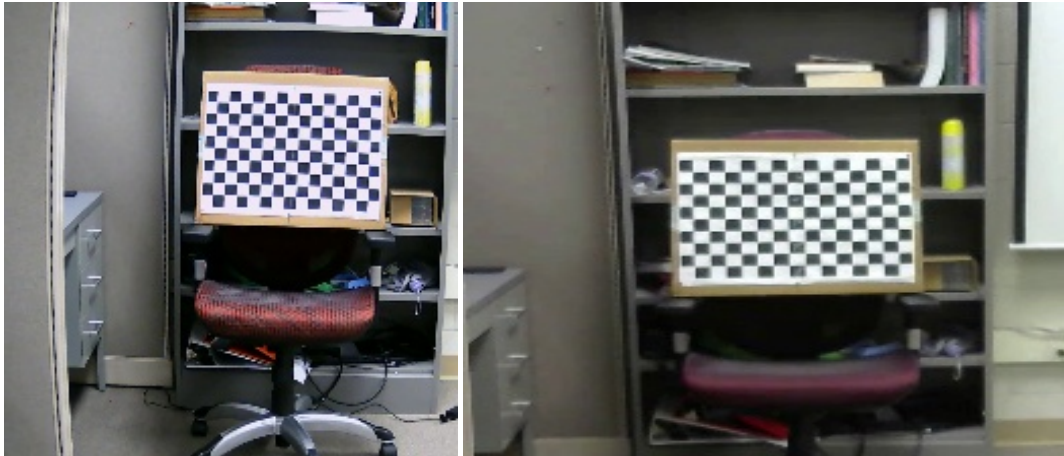
Fig. 22 Corresponding images from cameras 1 and 2 of the checkerboard dataset where the cameras are from different manufacturers.
