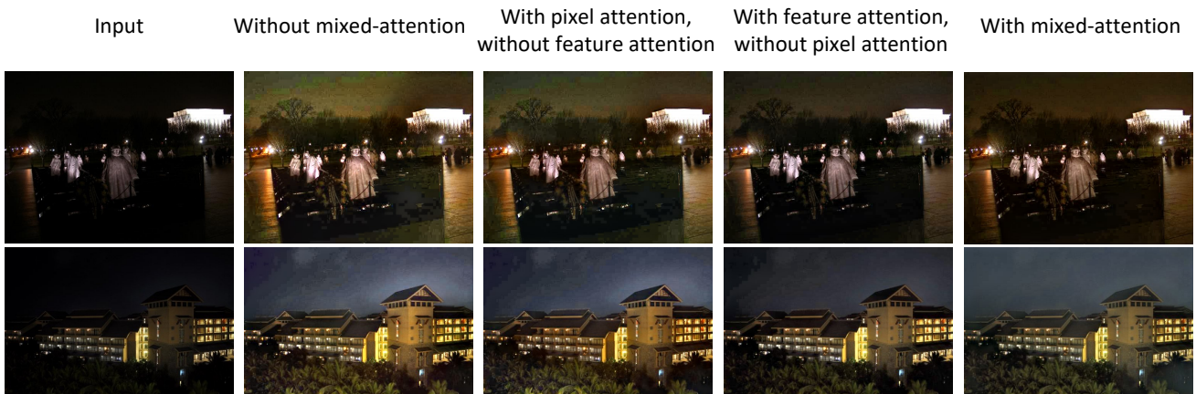
Fig. 6 Ablation study. Visual comparison of the results on the no-reference test dataset under each condition. In the absence of any of the attention modules, the images generated by the model are noisy and unnatural.
