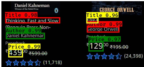
(b) Output: Multiple products with bounding boxes around product detail (e.g., book) without changes in website layout or location (URL)
