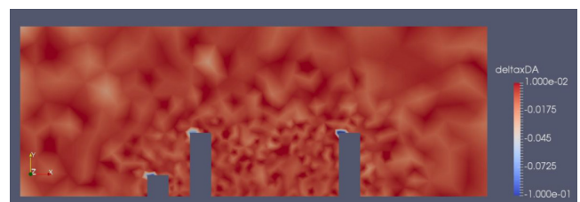
Fig. 10 Results of the VarDA algorithm with \tau=295 EOFs for Pressure field.
