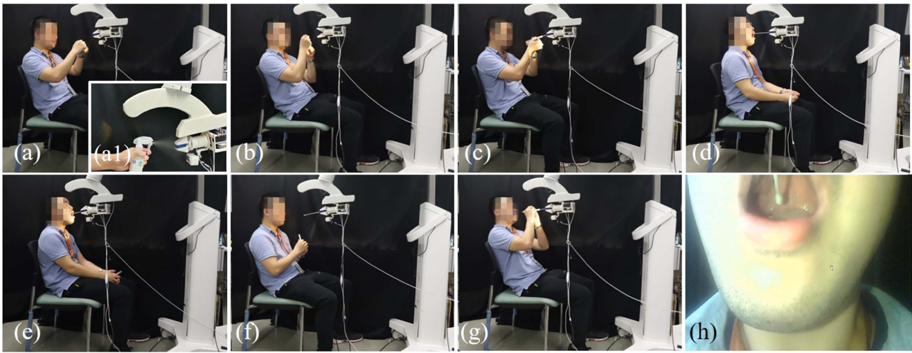
Fig. 14. Human user OP sampling demonstration. (a-a1) Sampling preparation and TSS hand can be directly sprayed by alcohol due to its waterproof feature. (b-c) Human-assisted swab replacing. (d) Swab insertion into the human mouth. (e) Swab teleoperation for specimen collection. (f) Swab withdrawal after specimen collection. (g) Human assisted swab collection. (h) Terminal camera feedback when swab inserting into the mouth.
