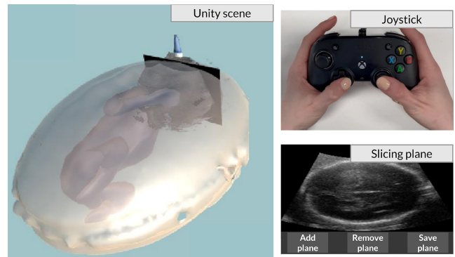
Fig. 4. Unity simulator for volume reconstruction, SP annotations, and automatic supervised data generation. Using the suggested commands, the clinician can visualize the slicing plane in an external window while controlling the probe with the joystick. Once the desired plane is reached, it can be saved using the “Save plane” button along with its 6D pose relative to the volume center.
