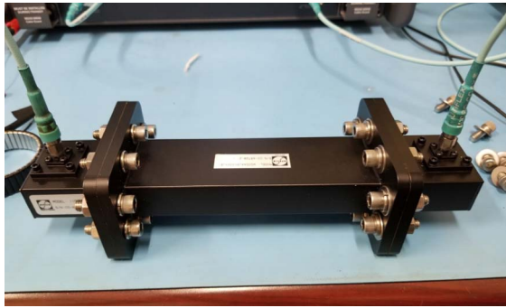
Fig. 21. Waveguide and adaptors under test in the Antennas Lab.
