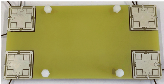
Fig. 21. Photograph of the geometry of 8 \times 8 MIMO antennas backed by a dielectric cover with the system circuit board of the 5G smartphone.
