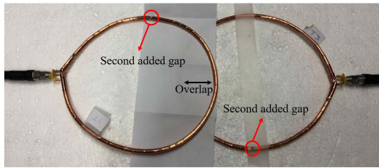
Fig. 8. (a) Chain of transmitting coils with optimal locations of the antenna ports. Sketched field spots (areas of the high magnetic field created every coil) practically do not intersect with the neighboring coils. By overlapping, one can obtain the complete decoupled situation between neighboring coils. (b) Chain with suitable locations of the antenna ports (especially for scanning fingers). (c) Chain with suitable locations of the antenna ports based on the HICs presented in [13].
