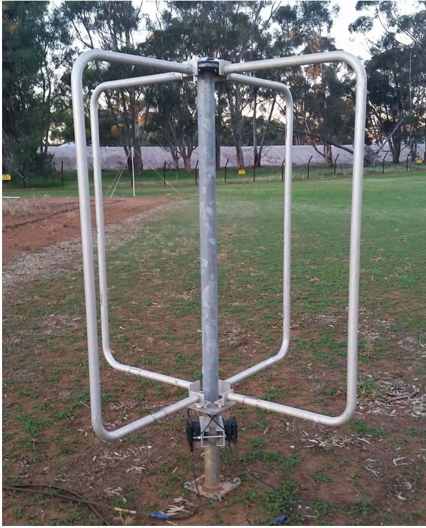
Fig. 1. Polarimetric receive antenna of the same type as used in this study.
