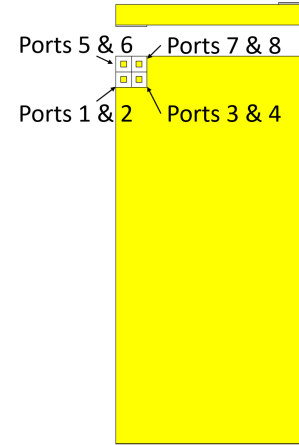
Fig. 5. Colocated array configurations, seen from front and top sides of the mobile phone chassis with one module on front- and one on back-side. Used in simulations (two discrete ports per element adding up to 16 ports in total).
